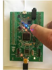
**Figure 3: STM32F4-Discovery board with a blinking LED example variant running.**
